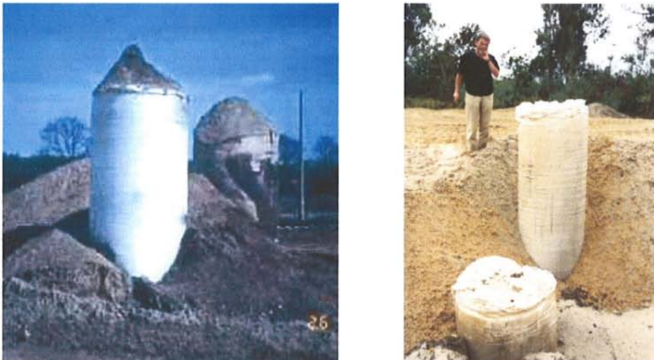
Figure 5. Test Ringtrac®-GEC constructed “in air” for demonstration in different testfields
