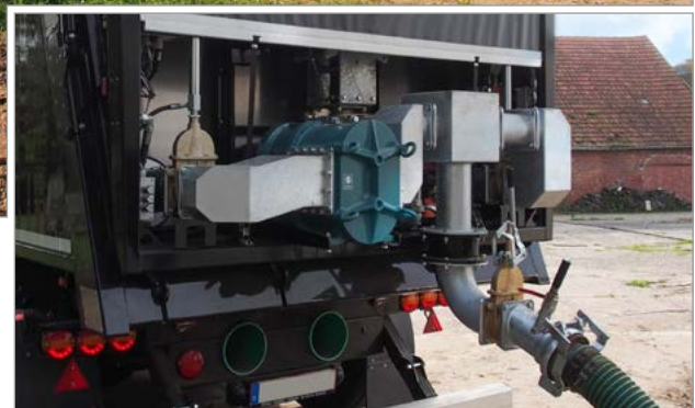
Rotary lobe pump with 6,000 U/min capacity, connected via swivel coupling.
