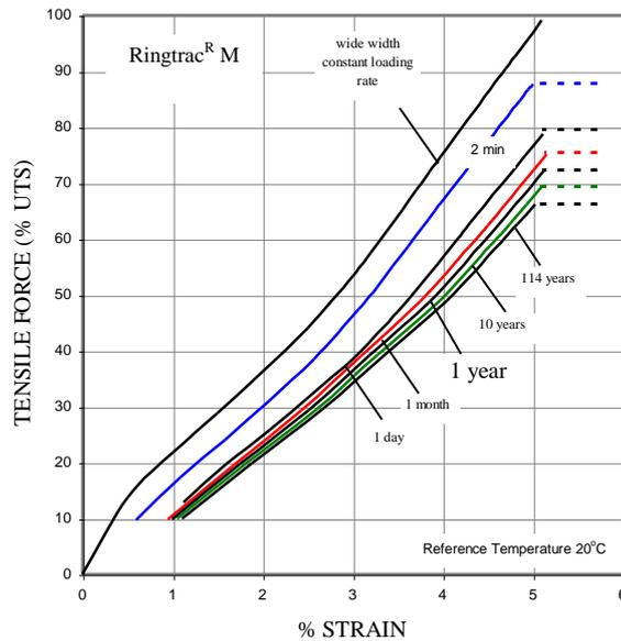
Figure 4. Isochronous curves for Ringtrac® M
