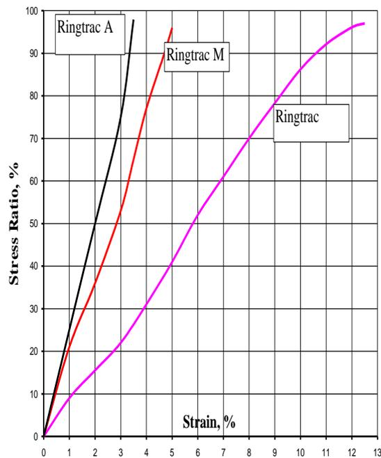
Figure 3. Initial Stress /Strain curves for different types of Ringtrac®
