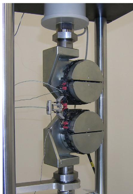
Fig. 5. Test set-up showing one thread (warp direction of the geogrid), clamping arrangements, extensometer (in the middle) and three thermocouples.
