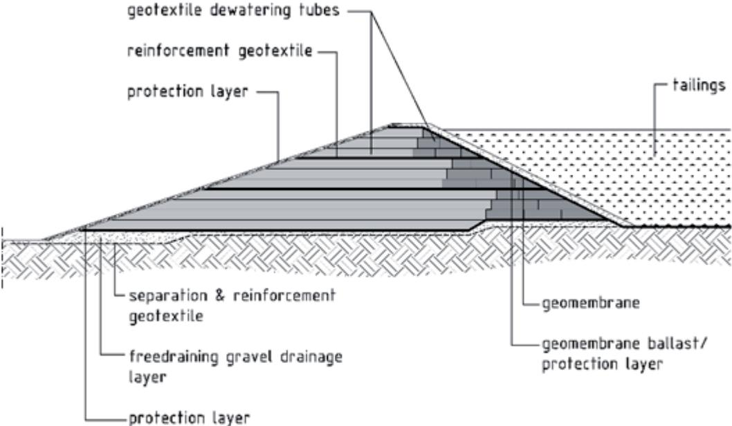
**Figure 4. Construction Concept: Dewatering tube tailings dams**
