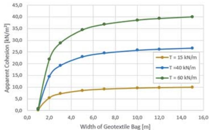
**Figure 6. Apparent cohesion calculated using Eq. 1 depending on width of geotextile bags, H = 2,0 m.  $\phi' = 20^\circ$**
