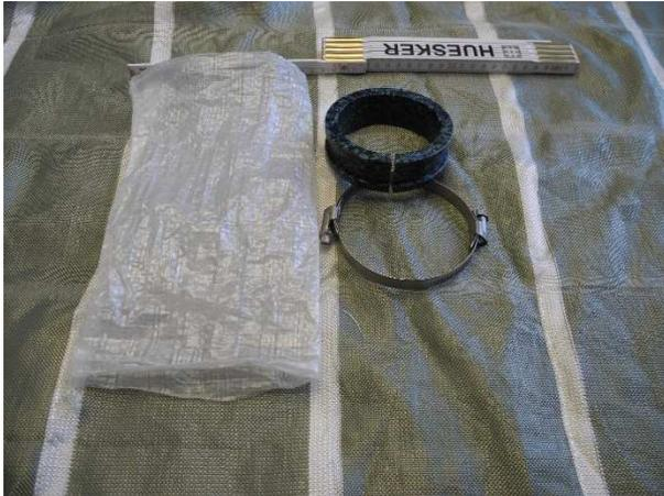
Illustration 1: Materials for installation of inlet (folding rule is not included)
