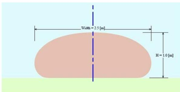
**Fig 10.** Cross-section of geotextile tube according to GeoCops
