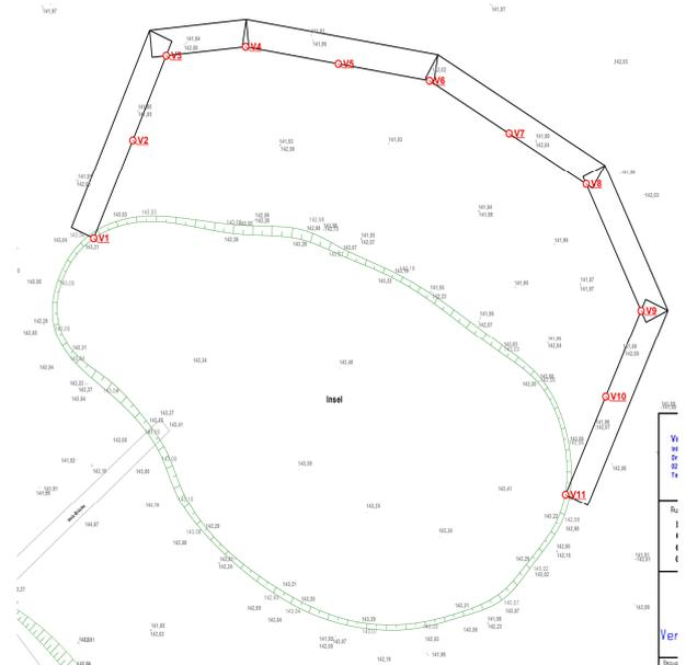
**Fig 11.** Layout plan of the tubes for the island reclamation area
