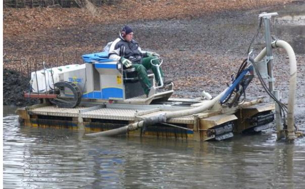
Fig 7. Amphibian dredging device
